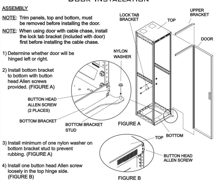
5) Install door onto bottom bracket stud, and holding door, install upper bracket stud to top of door. (FIGURE A) As an assembly, slip the upper bracket, with door attached, under the head of the loose screw on the top hinge side. Now install the second screw in the
